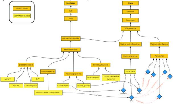
Figure 10: Taxonomy of materials models and relations used to specify the computational models used for the demo number 1.
