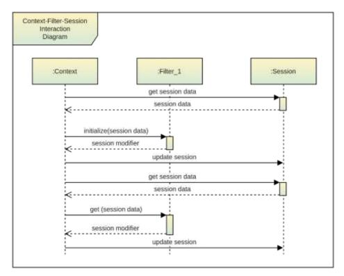
Figure 4. Context-filter-session diagram showing the communication between a context class, a filter, and the session.
