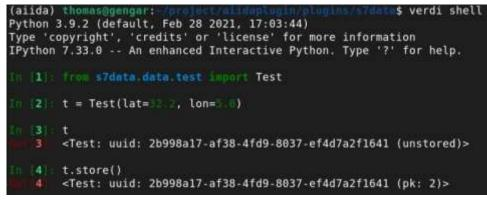
Figure 6. Example: Using a generated AiiDA plugin to instantiate a Data Node generated from a DLite/SOFT Entities.
